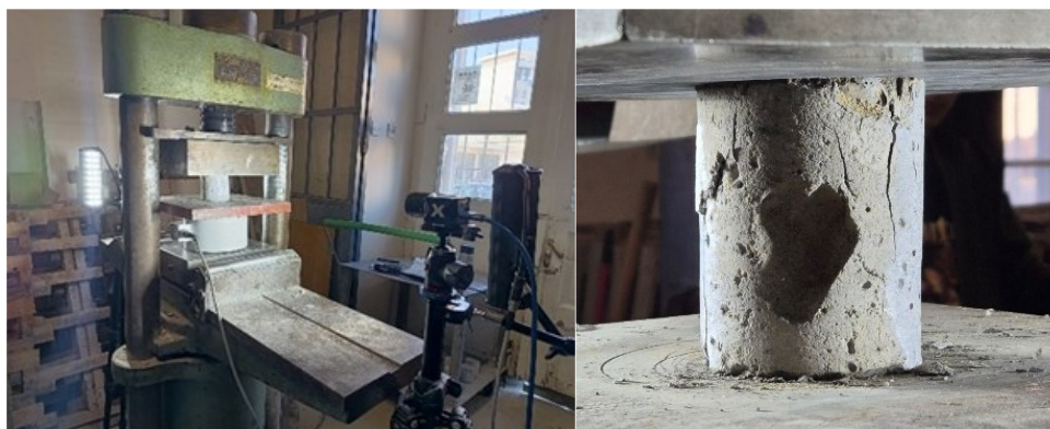
Figure 1. Testing experimental setup and one of the cracking patterns of the specimen
