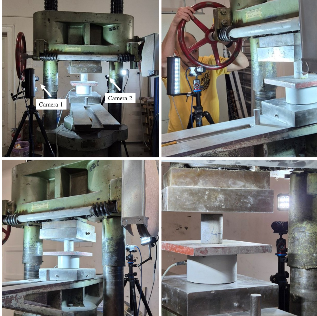
Figure 2. Experimental setup for uniaxial compression testing combined with DIC strain monitoring
